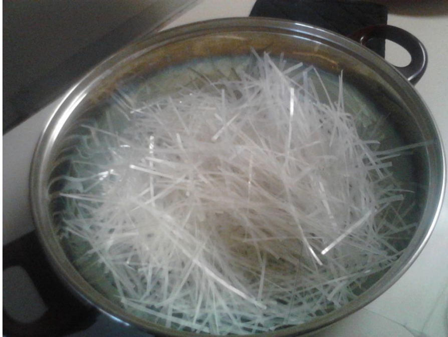
Figure 3.8: Shredded PET Fibers Source: Author
