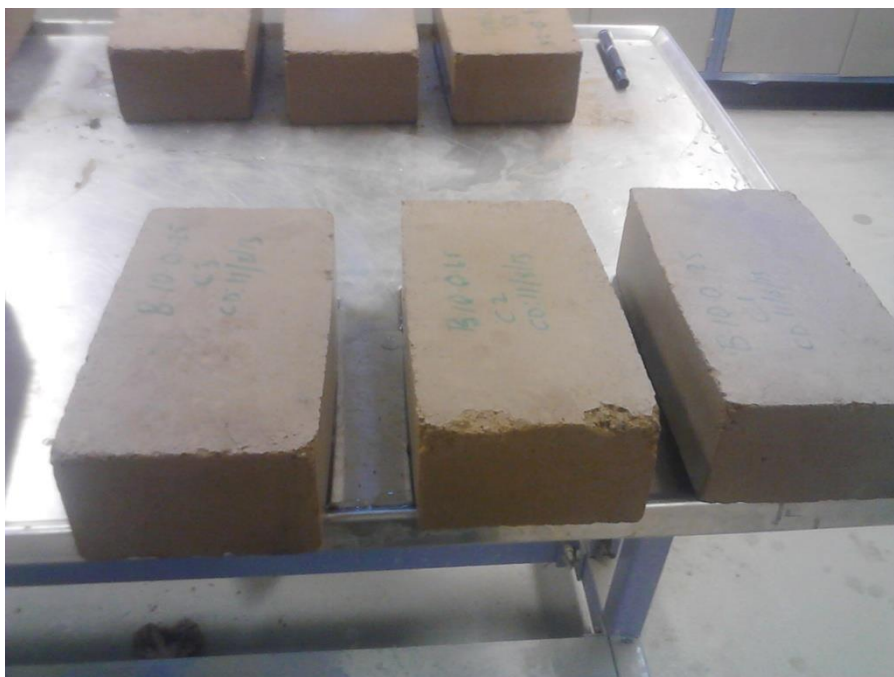
Figure 6.6: Submerged 10% stabilized earth blocks after 24hr
