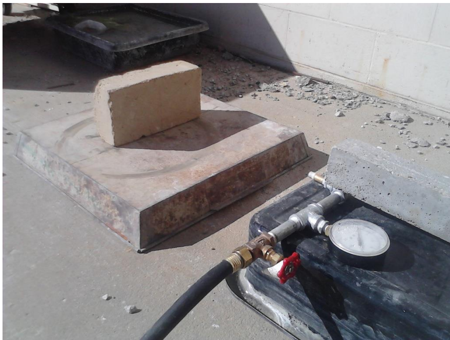
Figure 6.13: Surface penetration test set-up
