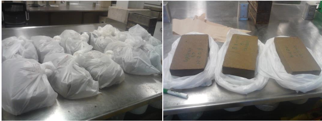
Figure 3.11: CSEB in Plastic Sheeting Source: Author
