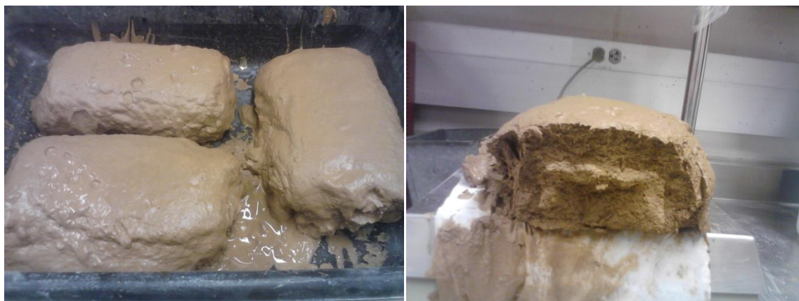
Figure 4.1: Submerged compressed earth blocks after 15mins Source: Author
