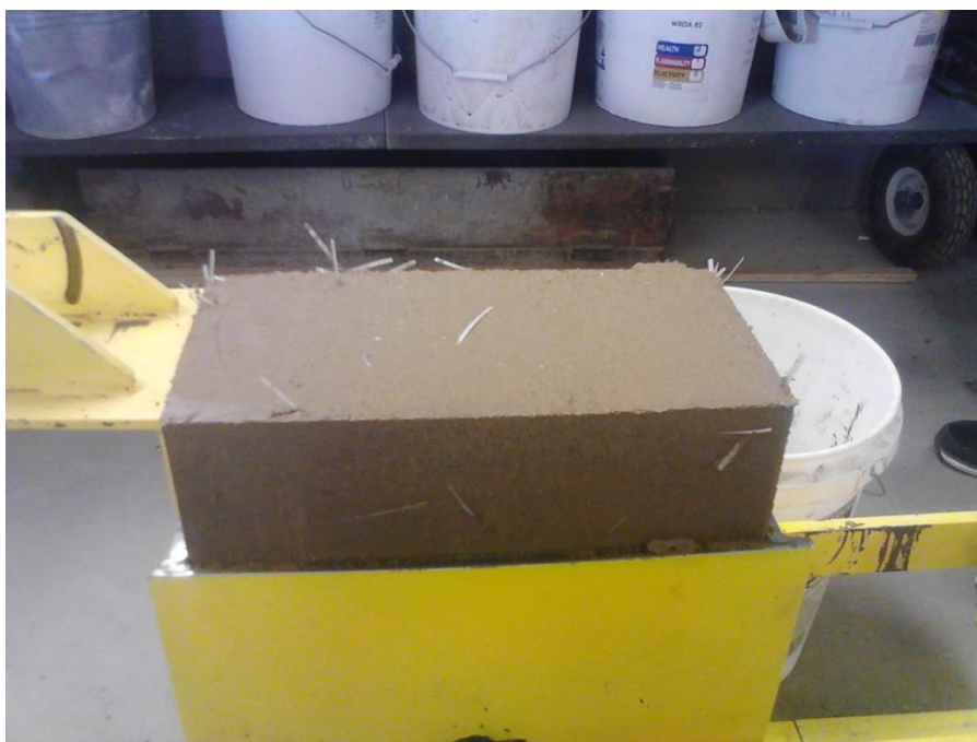
Figure 3.10: Cast Fiber Reinforced CSEB Source: Author
