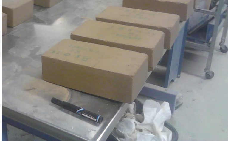
Figure 6.4: 8% stabilized earth blocks after 24hrs submersion
