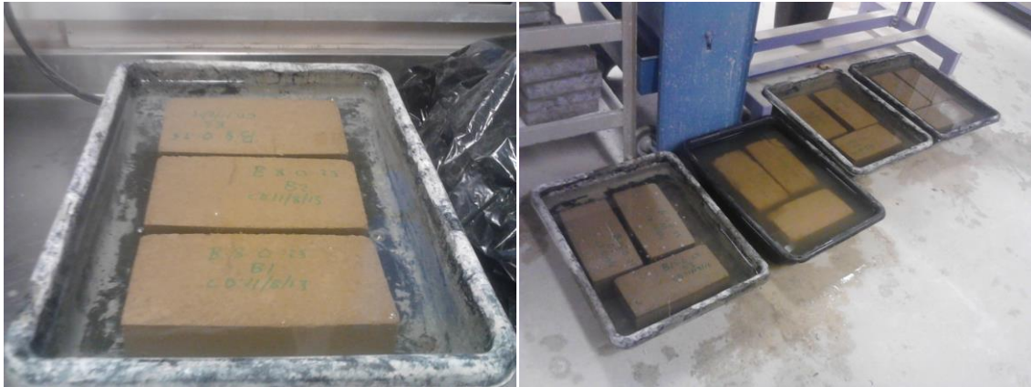
Figure 3.13: Submerged Blocks Source: Author
