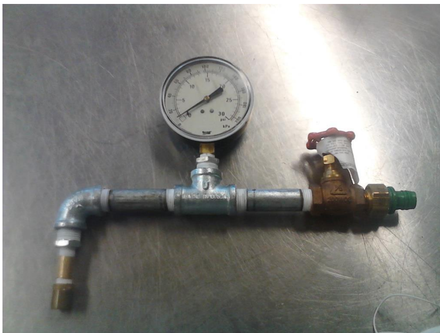
Figure 3.14: Pressure Gauge with Nozzle set up Source: Author
