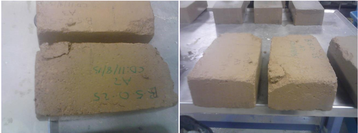
Figure 4.2: After 24hr submersion of the 5% stabilized blocks Source: Author
