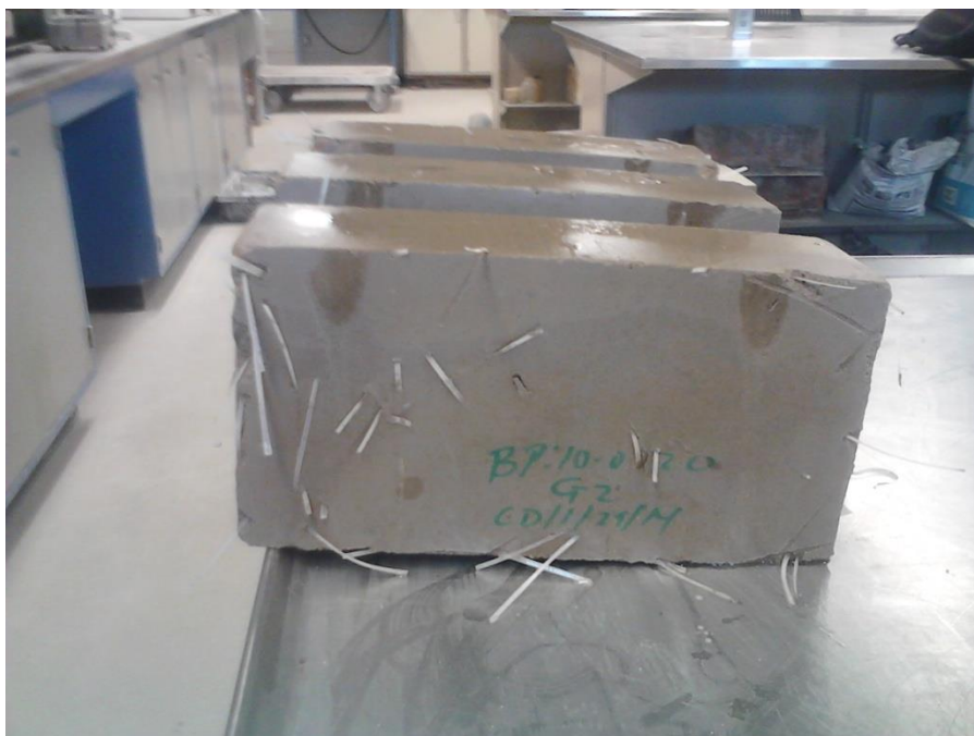
Figure 6.10: Absorption rate of 8% stabilized CSEB with PET fibers
