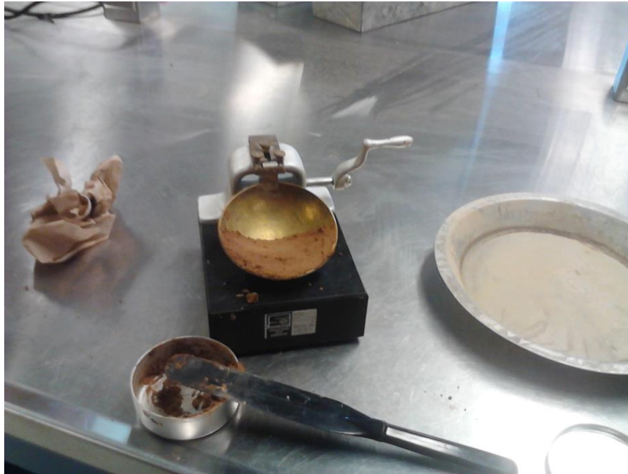
Figure 3.2: Casagrande Device Source: Author
