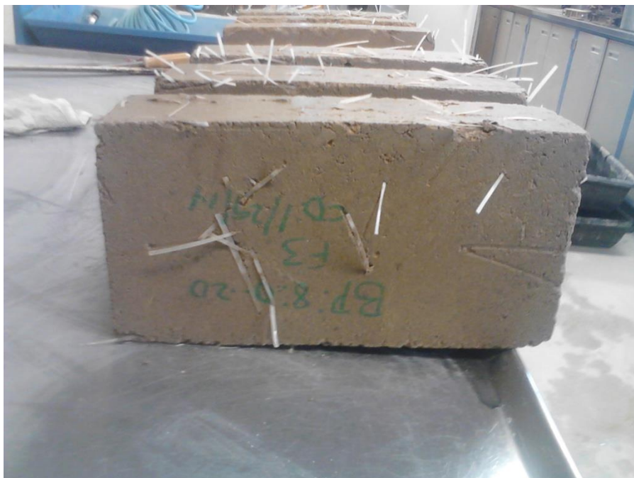
Figure 6.10: Absorption rate of 8% stabilized CSEB with PET fibers
