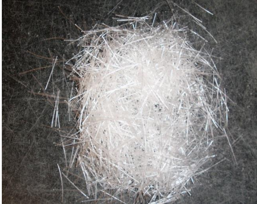
Figure 2.9: Polypropylene Fibers Source: (Donkor, 2013)
