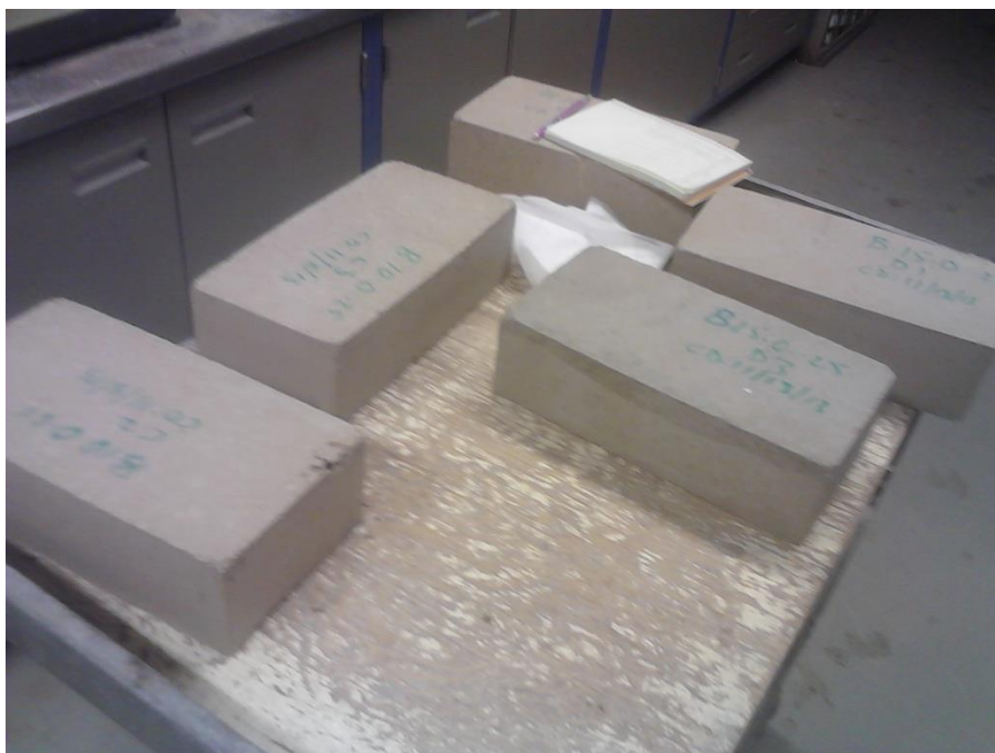
Figure 6.8: Submerged 15% stabilized earth blocks after 24hrs
