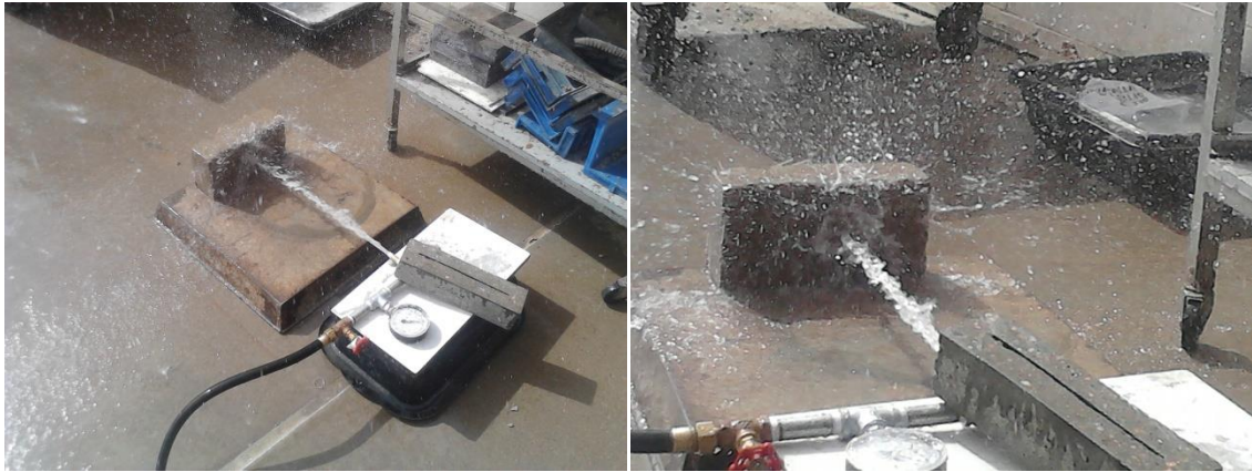
Figure 3.16: Spray test in progress Source: Author
